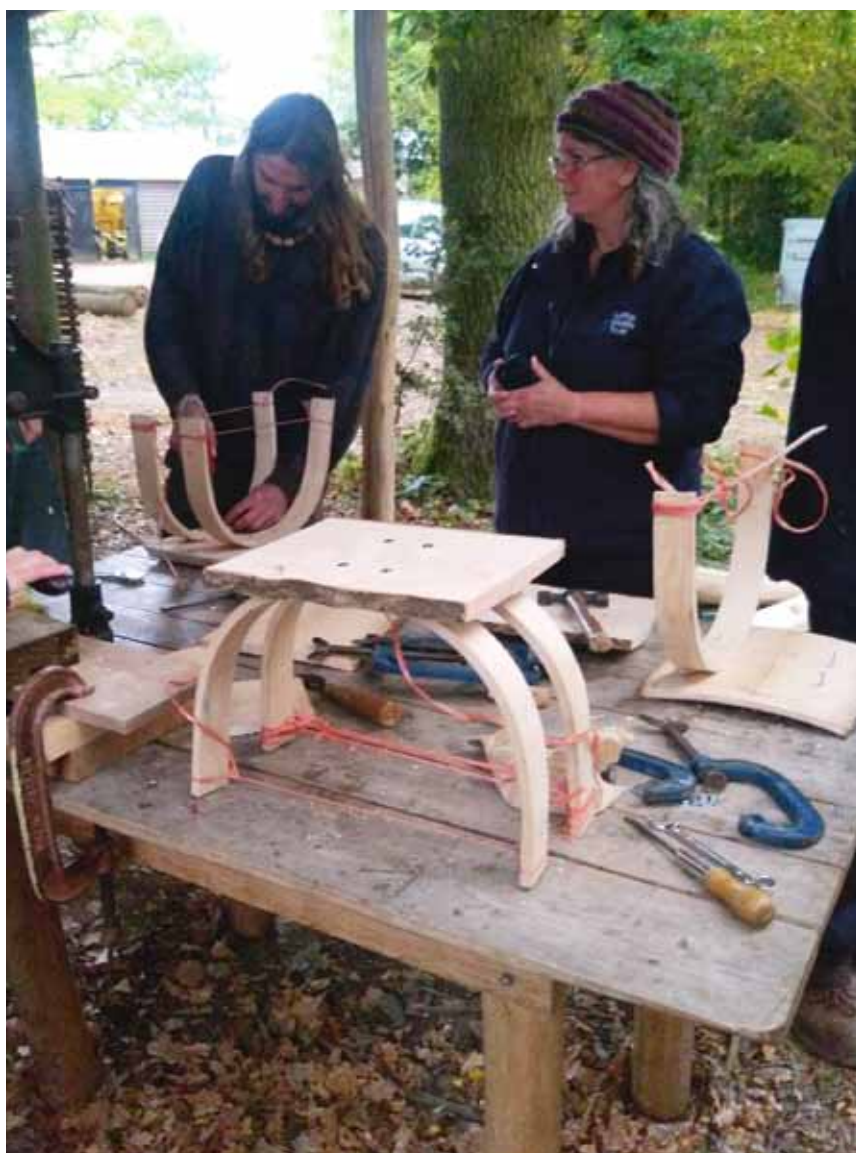
Attaching the legs to the finished stools
