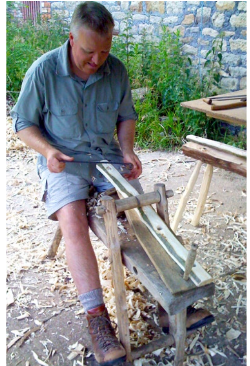
Using a draw knife with dropped handles to shape a billet on a shave horse.
