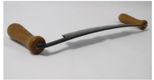
Svante Djarv draw knife, with handles cranked down, a straight edge, and curved blade.
